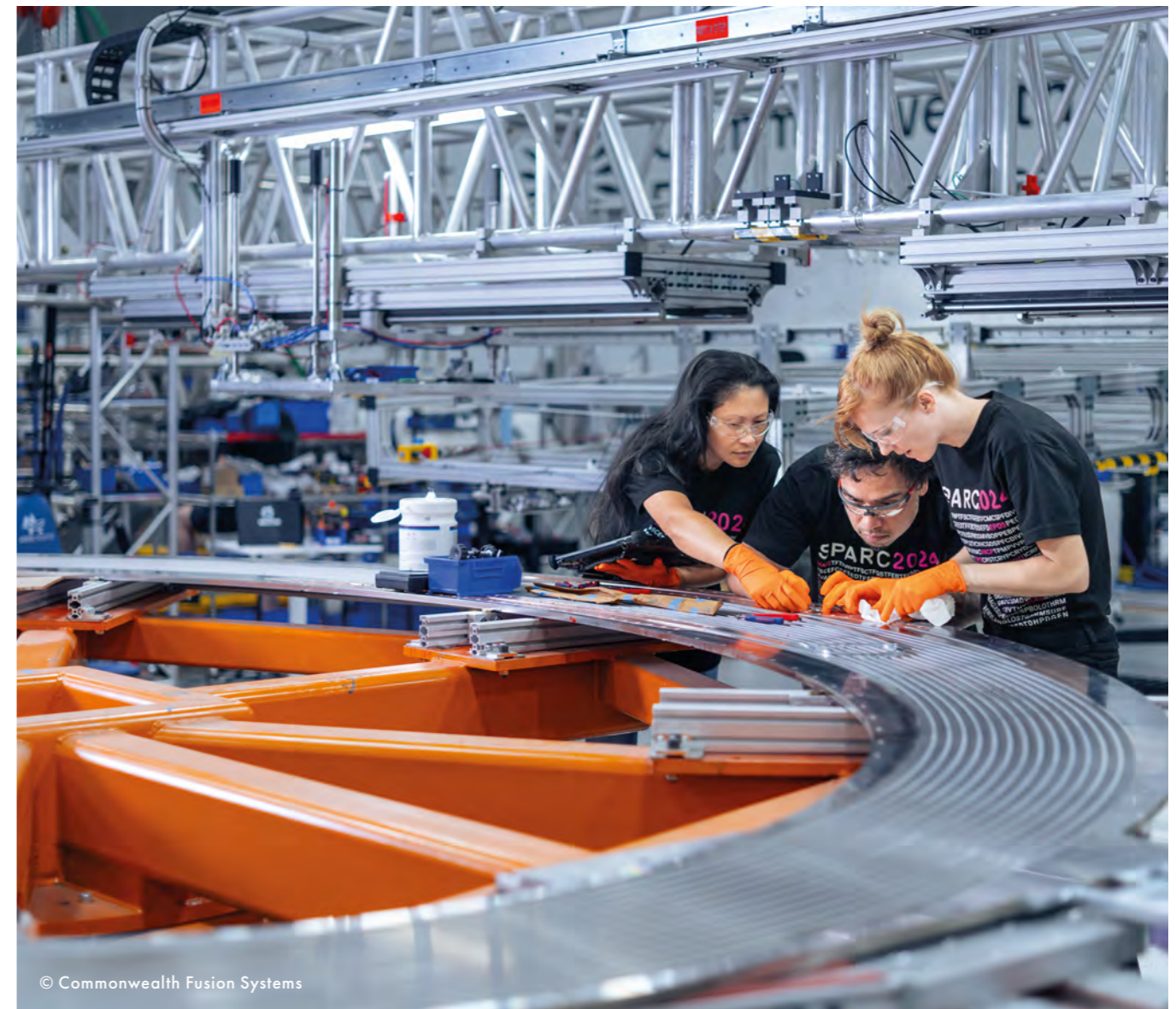
CFS employees work on a toroidal field magnet in the CFS Magnet Factory in Devens, Massachusetts.
